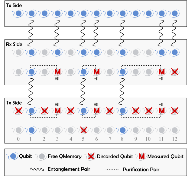
FIGURE 2. Pictorial representation of raw entanglement distribution and one step of entanglement distillation. In this example, the transmitter attempts to share 13-qubits, where each of them is part of a different Einstein–Podolsky–Rosen (EPR) pair. The receiver successfully detects seven qubits among the 13 transmitted ones. It groups three pairs for distillation, performs it, and discards the unpaired one. Finally, it sends the information about which qubit has to be kept and measurements to the original transmitter. Concluding the distillation procedure in this example, we have two EPR pairs in position 1 and 8 of the user’s respective quantum memories.
